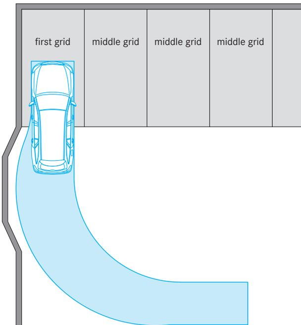
According to GaVo for Baden-Württemberg (07.07.1997/26.01.2011): For parking places with a 90° arrangement at the end of the driving aisle, the entrance width must be min. 275 cm.
