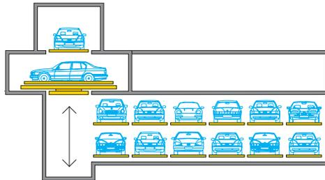
If there is an integrated turning device on the vertical lift, the cars can be rotated either in the transfer area or on an intermediate level, depending on the design of the building. (For details of the dimensions with turning device please contact WÖHR.)
