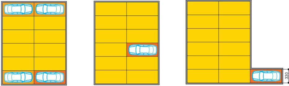
The vertical lift can be arranged at all four corners of the system. Special solutions with a vertical lift arranged at the front of the system or amongst the parking spaces can be constructed.
