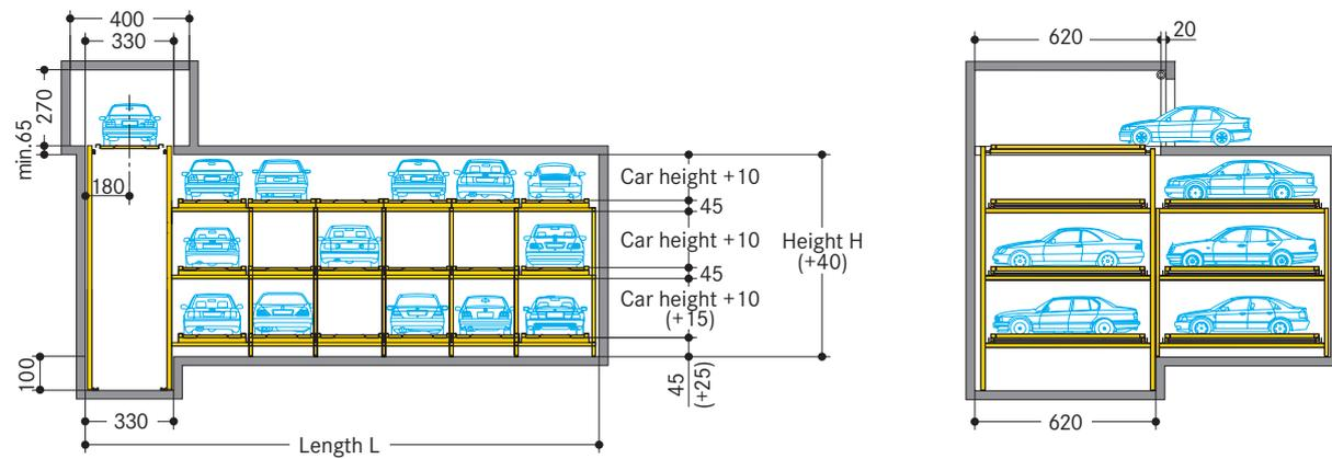
( ) Dimensions in brackets with turning device in the lowest level
