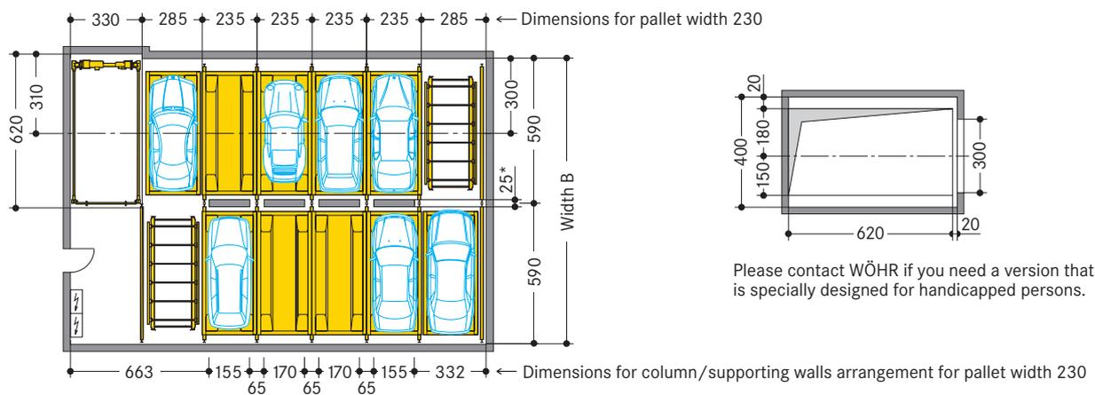
\* if the column/supporting walls width of 25 cm (minimum width 15) is changed, »width B« changes as well
