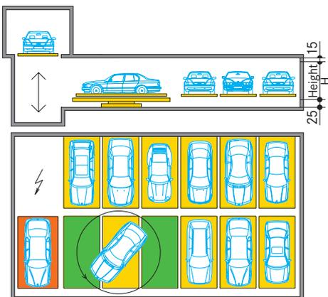
If the building offers no other alternative, the turning device can also be accommodated at the lowest parking level. (For details of the dimensions with turning device please contact WÖHR.)
