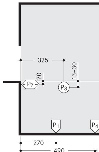
Bearing loads are transmitted to the pit floor by base plates of approximately 700cm<sup>2</sup>, fixed by heavy duty anchor bolts to a depth of approximately 10–12cm. Base plate thickness min. 18 cm. Concrete quality according to the static requirements of the building, but for the dowel fastening we require a concrete quality of min. C20/25. When fixing to waterproof concrete floors chemical anchors are employed (to be advised by Wöhr).
