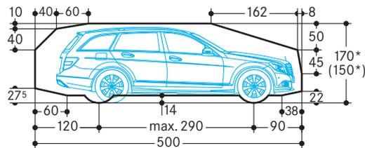
\*The total car height includes roof rail and antenna fixture and must not exceed the mentioned max. height dimension.
